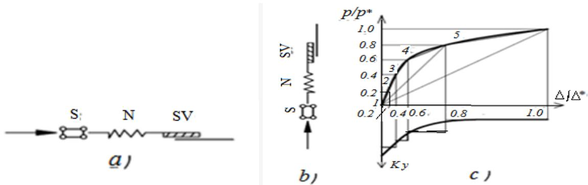
**Figure 8. Mechanical model of compression of the soil taking into account the structural element in the side (a) end (b) surfaces of the piles. Dimensionless curve pressure – lateral displacement (pressure – vertical offset) and a variable coefficient of stiffness of the soil correspond to the model (c).**
