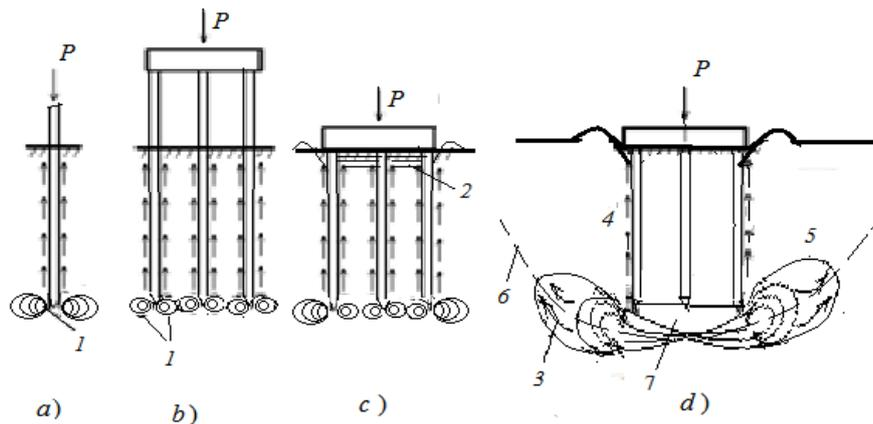
**Figure 5. The active region constrained deformation of soil from variable loads: a) single pile; b) high pile grillage; c, d) low-pile grillage**
