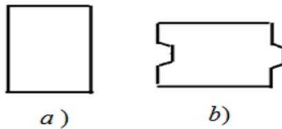
Figure 3. Cross section 2 piles with different cross-sections with the same perimeter
