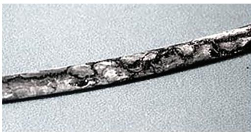
Fig. 1. Tracking erosion of CC close to:
