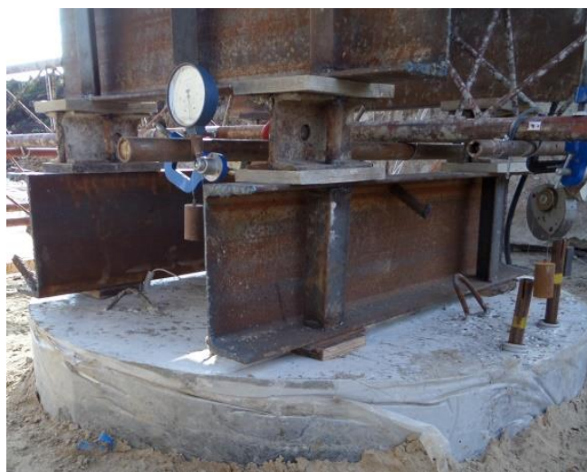
Figure 4. System of load transmission on the stamp surface
