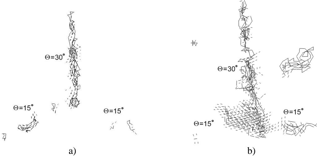
**Fig. 3.** Atomic displacements in projection on XY plane (depicted by segments) near the triple junction of  $<111>$  tilt boundaries with  $15^\circ$ ,  $15^\circ$ ,  $30^\circ$  misorientation angles during computer simulation for 150 ps at temperature of 1500 K: a) the vacancies were not introduced into the starting computational block; b) 2 % of conditional vacancies was introduced. Displacements less than 0.7 Å are not shown.
