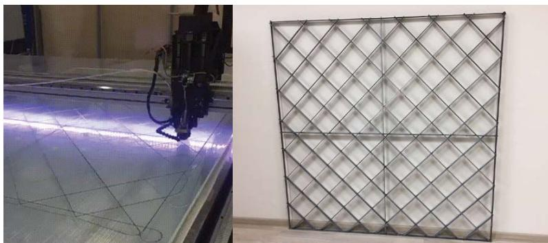
**Fig. 12.** 3D printed lattice structure.
