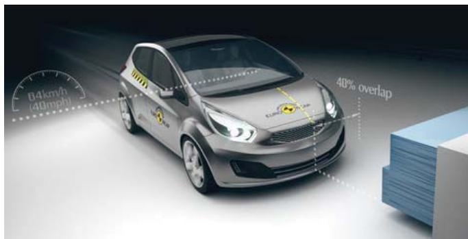
**Fig. 1.** Scheme of EuroNCAP frontal crash-test procedure.
