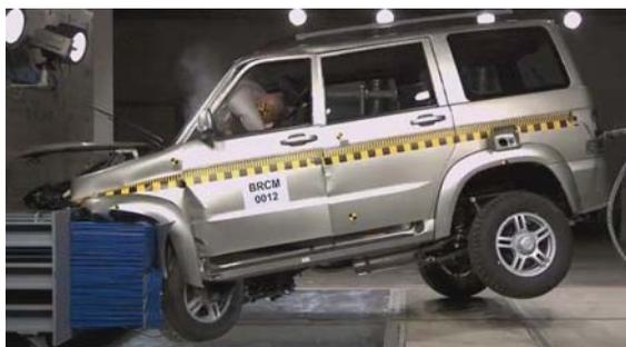
**Fig. 12.** Deformation in actual crash-test.
