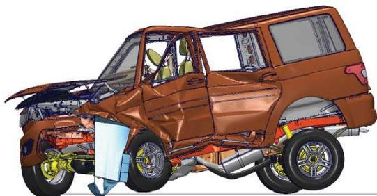
**Fig. 10.** Deformation with customer material models.
