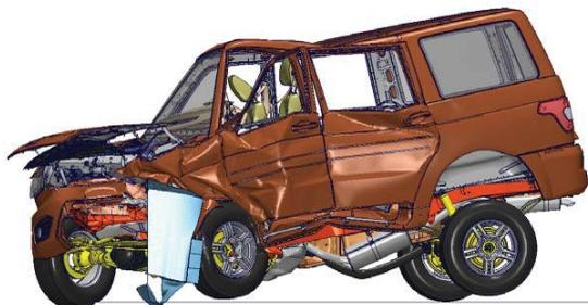
**Fig. 10.** Deformation with customer material models.
