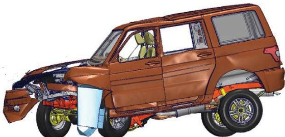
**Fig. 11.** Deformation with optimized material models.
