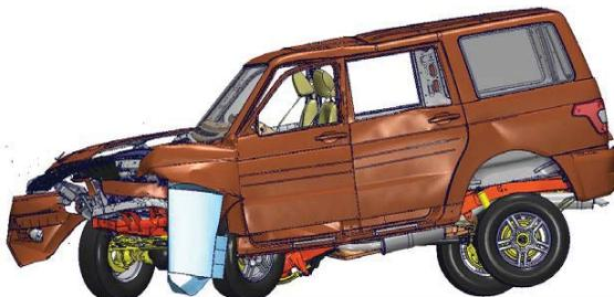
**Fig. 11.** Deformation with optimized material models.
