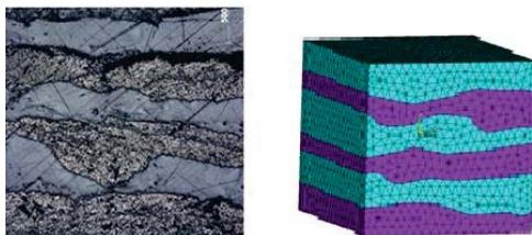
**Fig. 1.** Mesostructure of a three-component material and its FE model.
