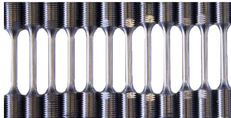
**Fig. 1.** Specimens for tensile test
