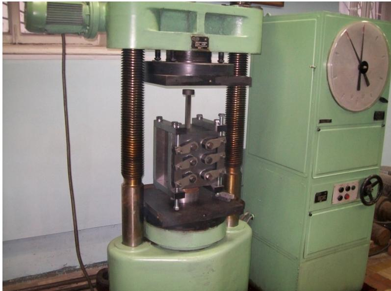
**Fig. 1.** Experimental equipment for ECAP.
