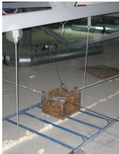
Figure 7. The load on the safety ropes
