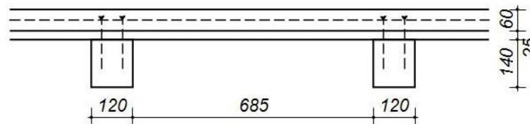
Figure 1. Layout scheme of the ceiling elements
