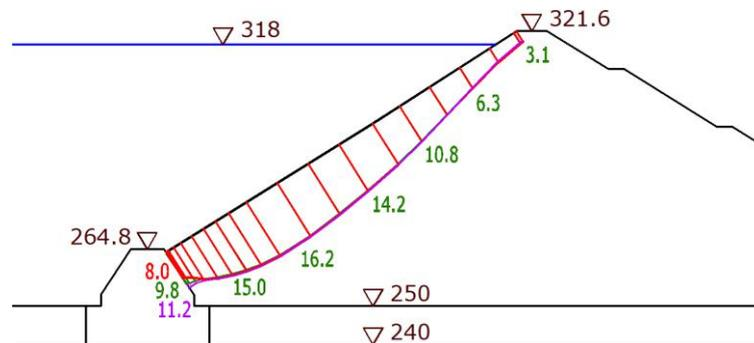
**Figure 3. Displacements of the dam upstream face in perpendicular direction (deflections, cm). The green color indicates displacements for Alternative 2, red – for Alternative 1, violet – for Alternative 3.**
