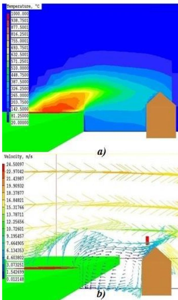
**Figure 2. The distributions of temperature a) and velocity b) near from the building**
