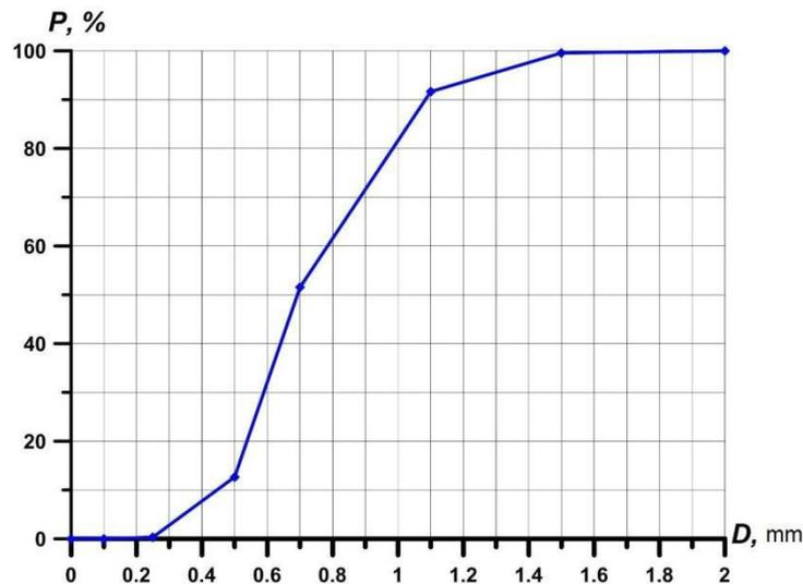
Figure 5. Model grain-size distribution of filter layer material
