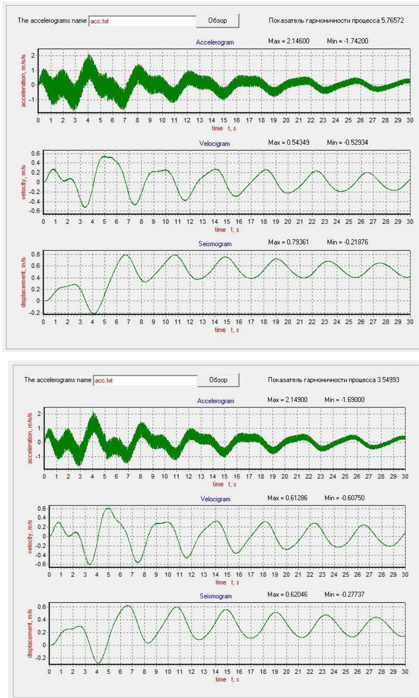
Fig.5. Oscillograms of artificial input for pPGA = 0.1 (on top) and pPGA = 0.6 (on bottom)
