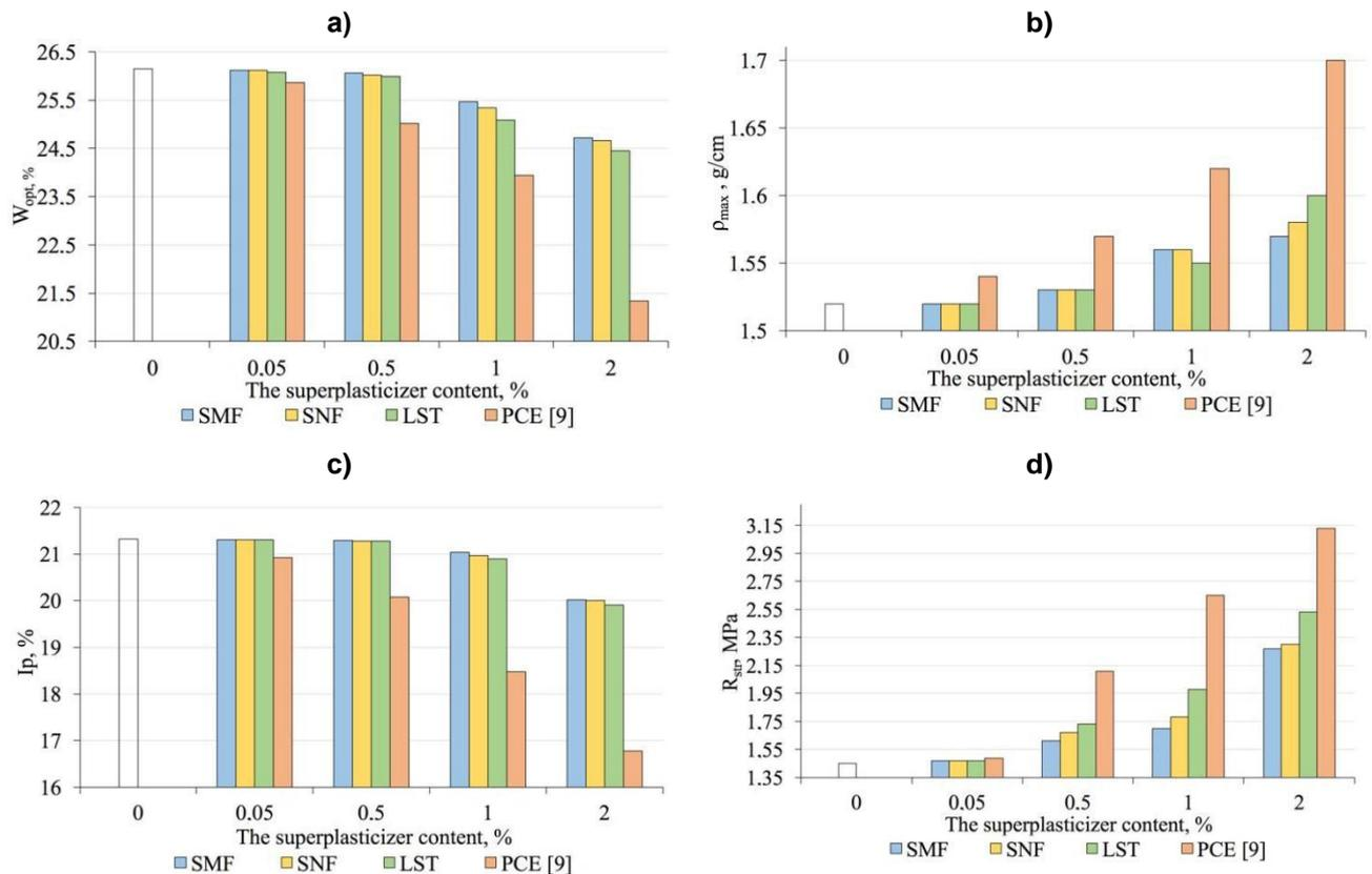
**Figure 2. Dependences physical and strength properties of bentonite clay of the dosage of plasticizing surface-agents: a) the optimum moisture; b) the maximum density; c) the plastic index; d) the ultimate compressive strength**
