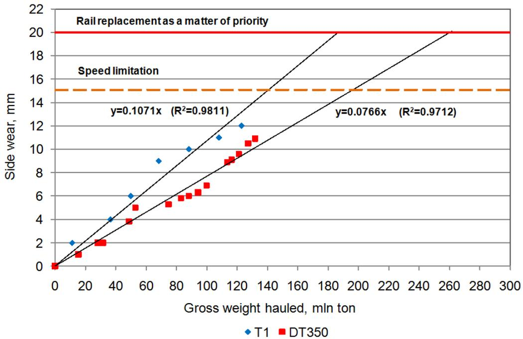
**Figure 8. The side wear of T1 and DT350 rails in a curve of radius 390 m (high rails)**
