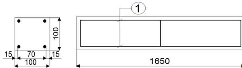
**Figure 2. Scheme of reinforcement of fibreconcrete beams:**
