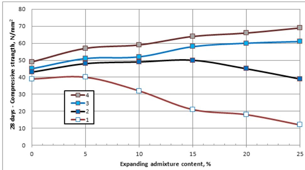
**Figure 3. The influence of expansion deformation constraint conditions on the strength under the concrete compression: 1 – without deformation constraint; 2 – uniaxial deformation constraint; 3 – biaxial deformation constraint; 4 – triaxial deformation constraint**
