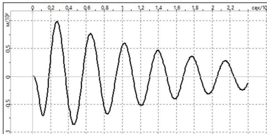
**Figure 10. Calculational vibrorecord of displacements in the middle of the span of the beam**
