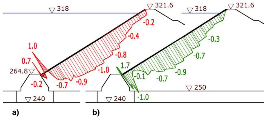
**Figure 5. Longitudinal stresses in the soil-cement bedding downstream face (MPa)**
