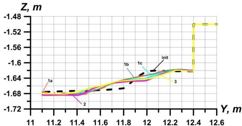
**Figure 13. Geometry of the central section of windward scour protection face after execution of tests 1a, 1b, 1c, 2, 3 for wave direction with angle  $90^\circ$  to a plane side of BGT "Prirazlomnaja" (— — — - initial geometry).**
