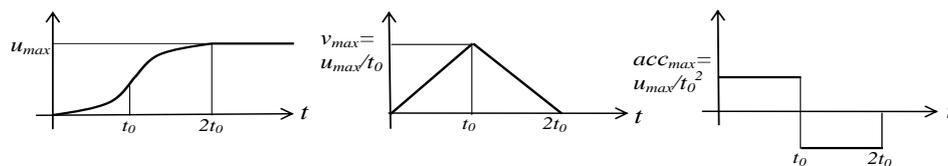
**Figure 1. Time charts of displacements, velocities and accelerations for the speed pulse**
