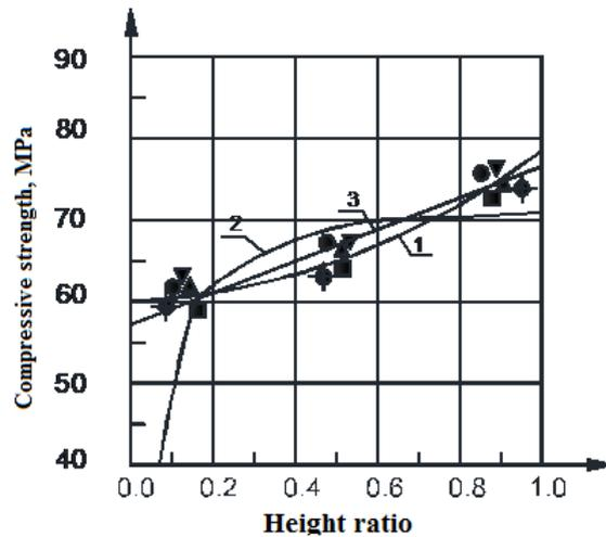
Figure 3. Comparison of mathematical relationships describing the patterns of change in the strength of centrifuged concrete
