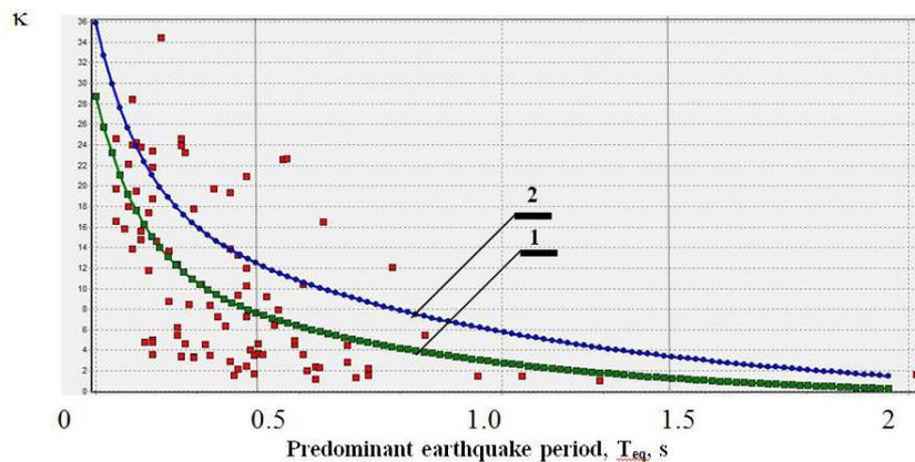
Figure 2. Dependence  $\kappa(T_{eq})$  obtained on the basis of the available records of real accelerograms.
