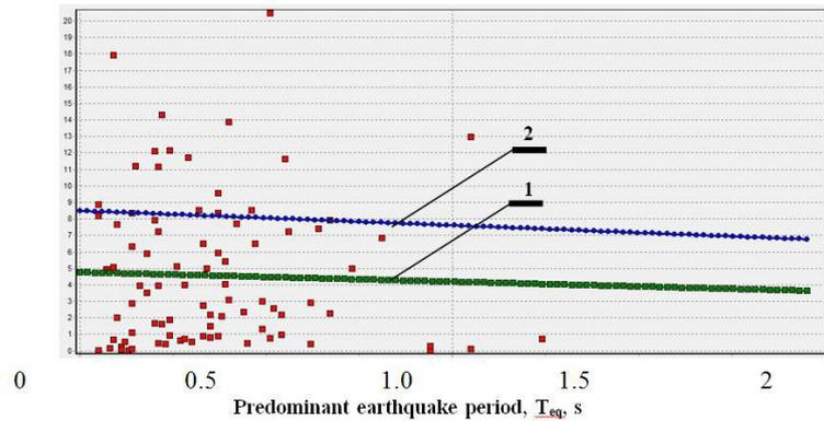
Figure 3. Dependence  $I_A(T_{eq})$ . 1 – average value; 2 –  $I_A(T_{eq}) + \sigma_I$
