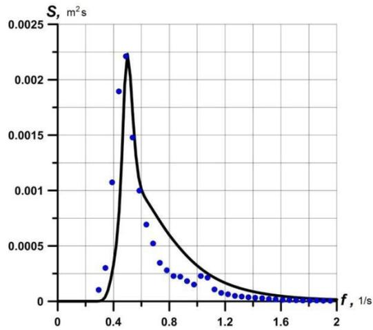
Figure 7. Wave spectrum for conditions of tests 1,2 with repeatability 1 times in 100 years
