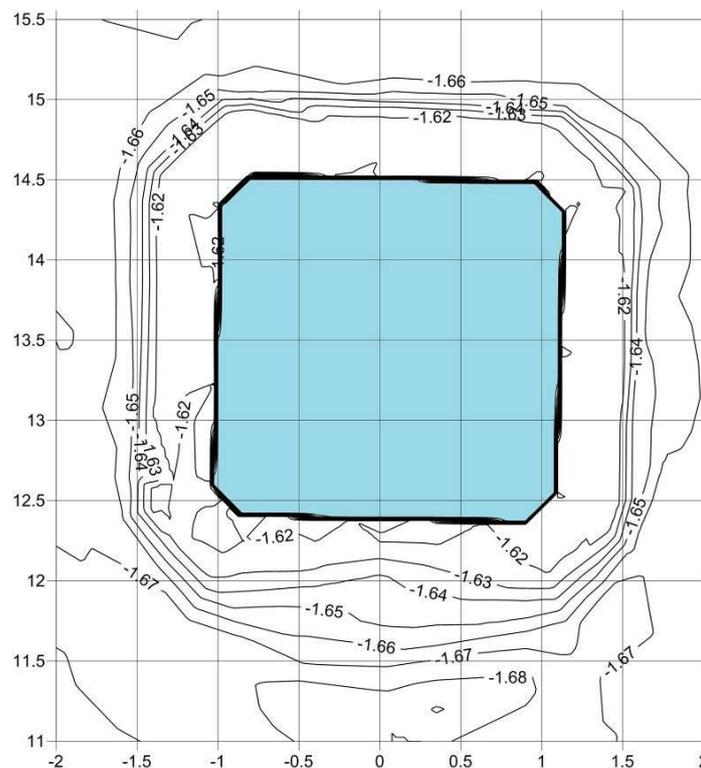
Figure 12. Plan of scour protection levels after execution of tests 1a, 1b, 1c, 2, 3 for wave direction with angle  $90^\circ$  to a plane side of BGT "Prirazlomnaja" (level  $-1.62$  m corresponds to the top level of scour protection before researches)
