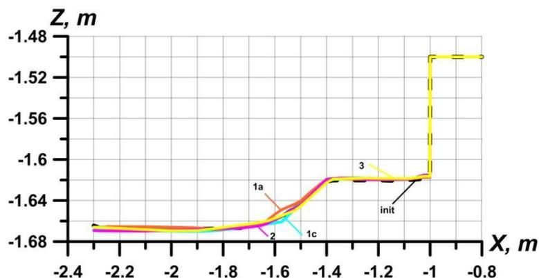
**Figure 14. Geometry of the central section of left side scour protection face after execution of tests 1a, 1b, 1c, 2, 3 for wave direction with angle  $90^\circ$  to a plane side of BGT "Prirazlomnaja" (— — — - initial geometry)**
