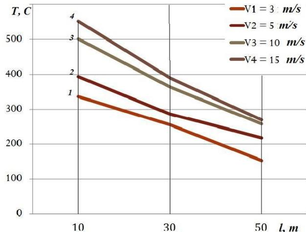
**Figure 3. The dependence of the temperature on the walls of a wooden house for different wind speeds (3-15m/s) for the different distances l (10-50 m)**
