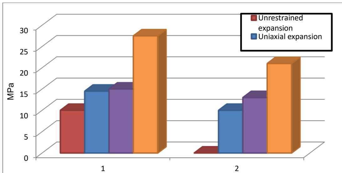
**Figure 4. The influence of constraint degree of the expansion process on the strength under compression, porosity and expansion pressure: 1 – strength under compression; 2 – pressure under stable expansion**
