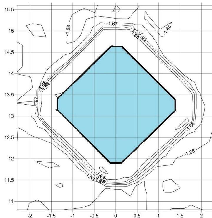
**Figure 17. Plan of scour protection levels after execution of tests 1a, 1b, 1c, 2, 3 for wave direction with angle  $45^\circ$  to a plane side of BGT "Prirazlomnaja" (level  $-1.64$  m corresponds to the top level of scour protection before researches)**
