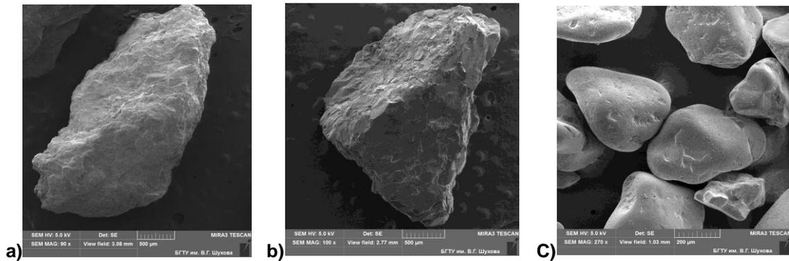
Figure 1. The grain: a – dropping out of quartzitic sandstone; b – dropout granite; c – natural sand
