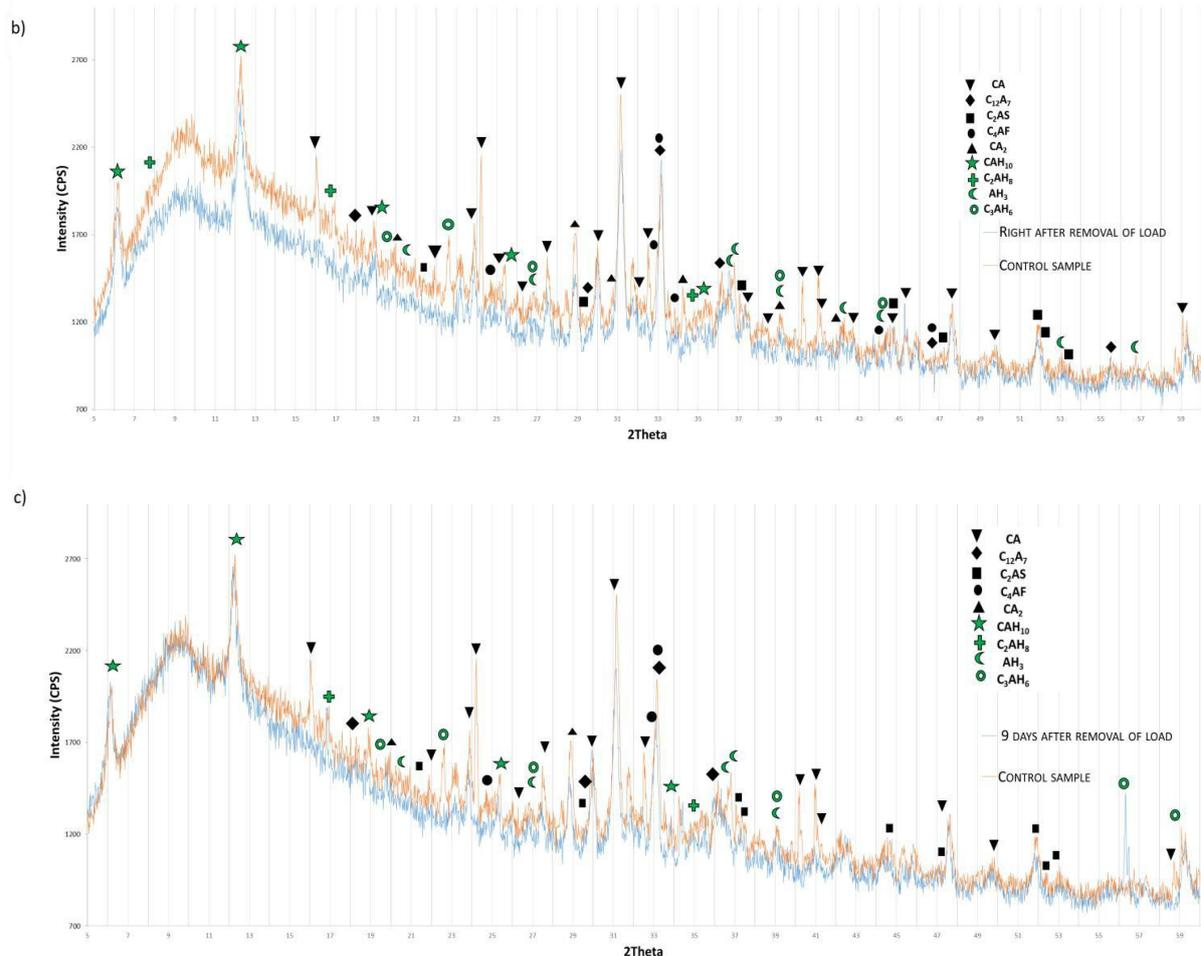
**Figure 2. X-ray diffraction patterns of the cement GC-50 before mixing with water (a), immediately after removal of the load (b) and 9 days later (c)**
