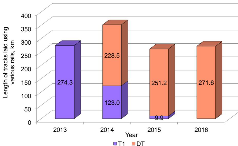
Figure 1. Annually laid volumes of T1 and DT rails at WSID
