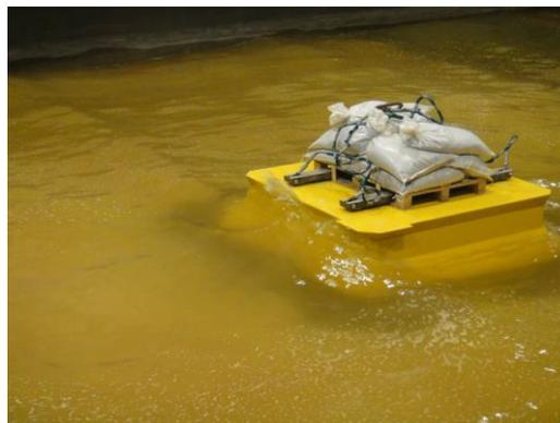
Figure 9. Interaction of waves with BGT during execution of researches for wave direction with angle  $90^\circ$  to a plane side of BGT "Prirazlomnaja" (view from windward side)
