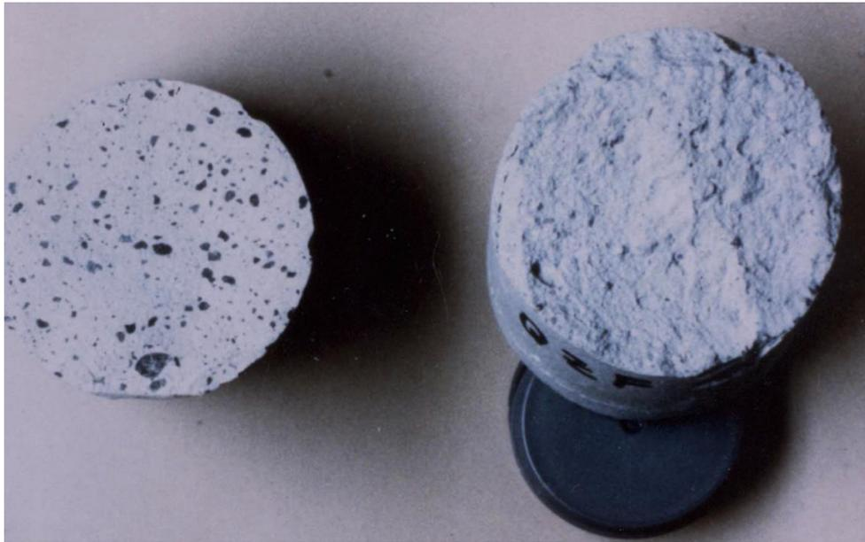
**Figure 5. The formation of black aggregates in the cement stone volume, hardening at isotropic deformation constraint conditions (left sample) and the absence of aggregates during hardening without deformation constraint (right sample) at an expansion potential capacity of 185 mm/m**
