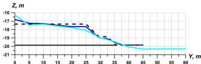
**Figure 18. Natural data on the changes of geometry of scour protection section located near to the center of North face of MIRP "Prirazlomnaja" - - - - a design profile, ———— a profile after building of scour protection in 2011, ———— a profile in conditions of 2016).**
