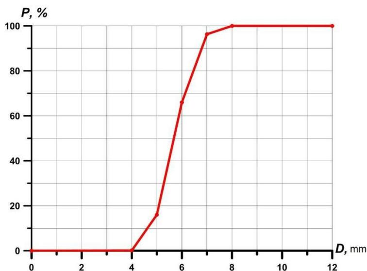
**Figure 4. Model grain-size distribution of protective layer stones**
