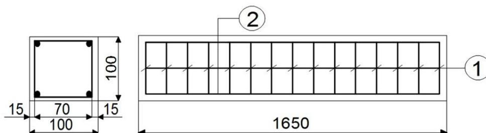
**Figure 1. Scheme of the reinforcement of ferroconcrete beams:**
