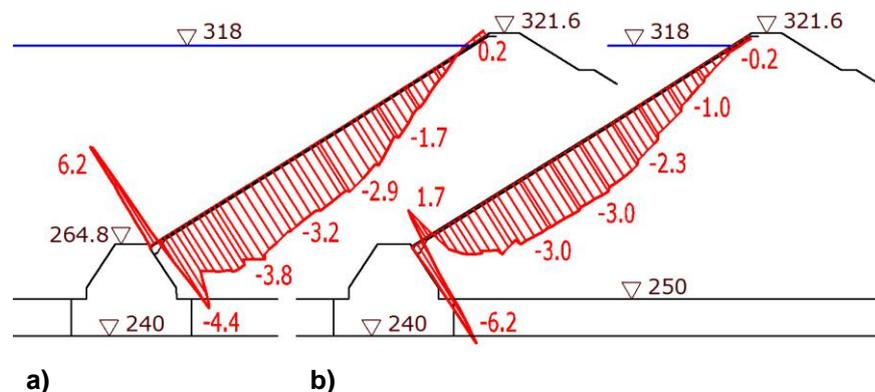
**Fig.6. Longitudinal stresses in the reinforced concrete cover (MPa) in Alternative 2**
