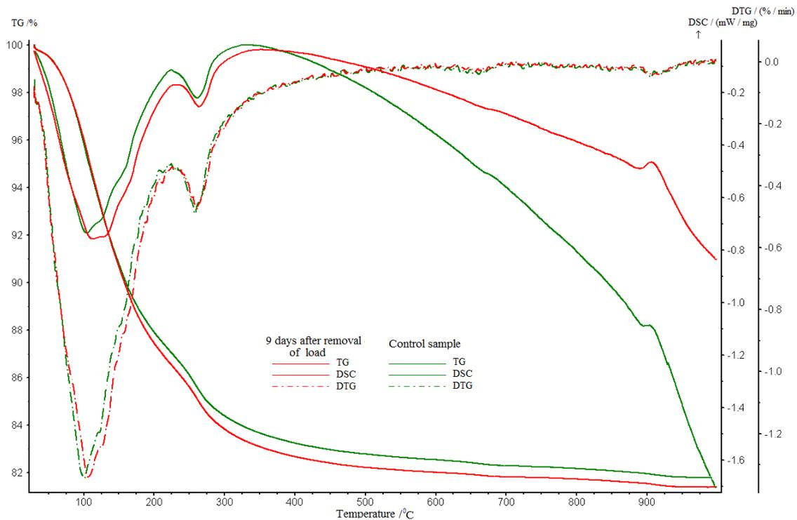
Figure 3. Comparison of the compressed and control specimens through differential thermal analysis 9 days after removal of the load
