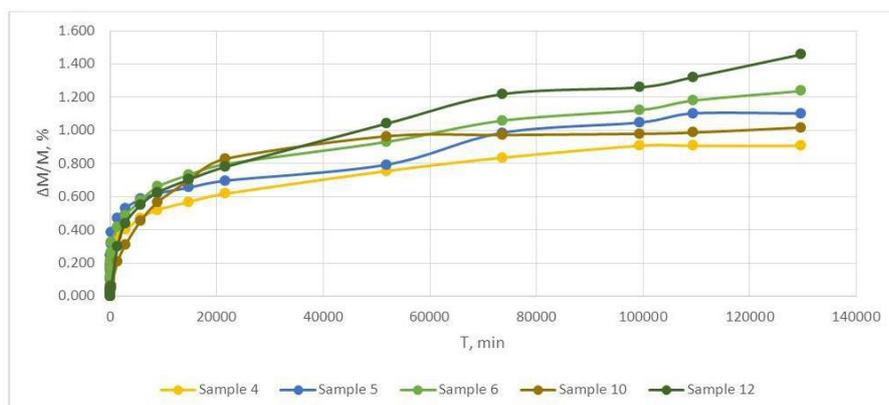
**Figure 3. Water saturation of 4, 5, 6, 10, 12 samples - time graph**
