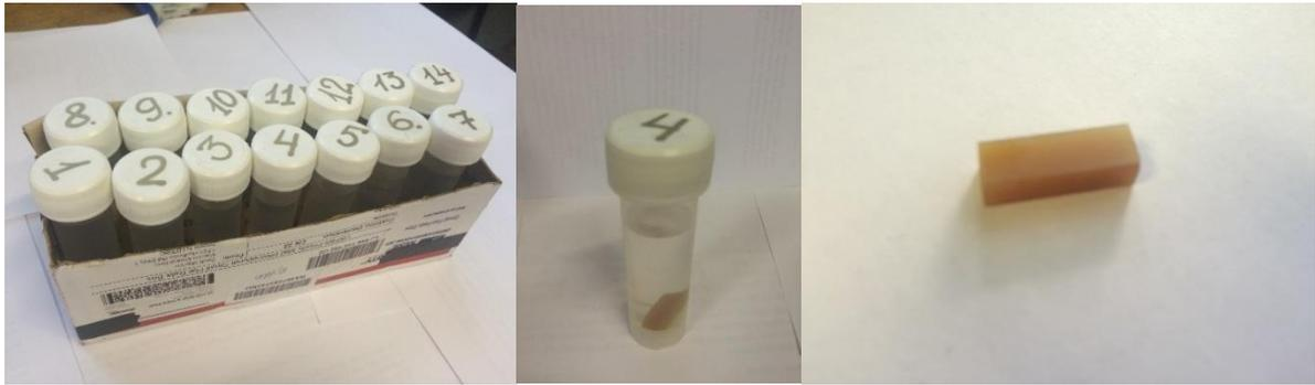
**Figure 1. Exposure of polymer compounds samples in water**
