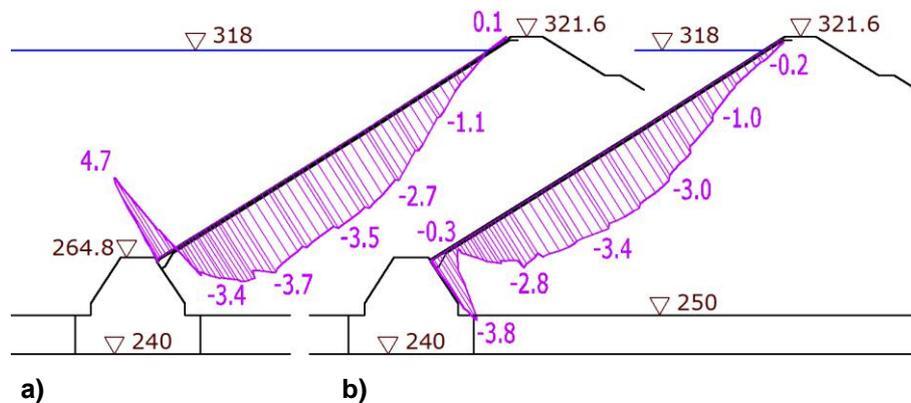
**Fig.7. Longitudinal stresses in the reinforced concrete cover (MPa) in Alternative 3
