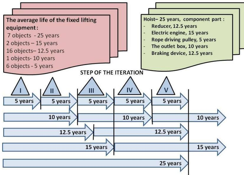
**Figure 2 Algorithm for ensuring the safety of components with a comparison of the lifetime of the elements of the elevator**
