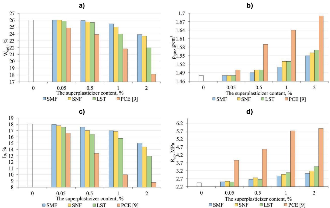
**Figure 1. Dependences physical and strength properties of kaolinite clay of the dosage of plasticizing surface-agents:**
