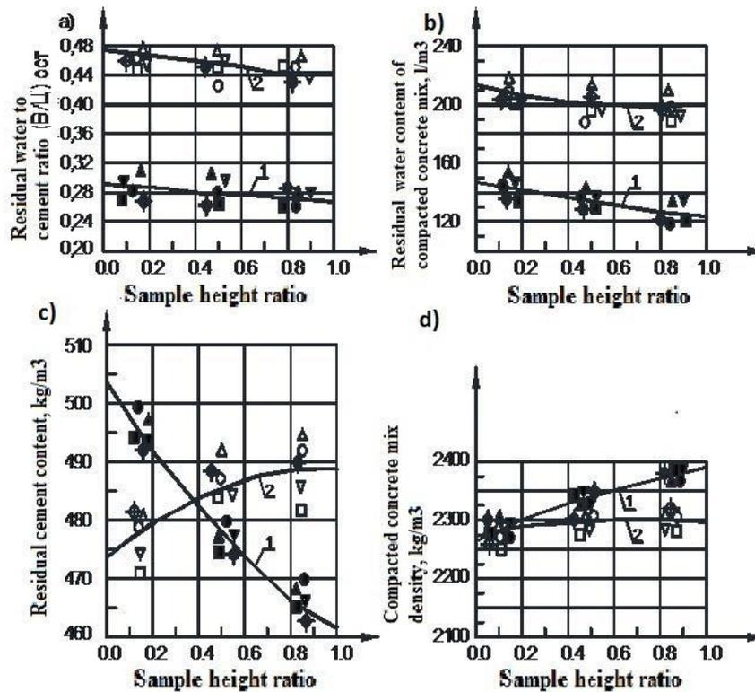
Figure 1. Variance of compacted concrete physical properties along a sample height (a – residual water/cement ratio; b – residual content of water; c – residual cement content; d – average density).
