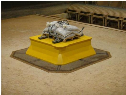
Figure 8. View on BGT model and scour protection before the beginning of experimental researches for wave direction with angle  $90^\circ$  to a plane side of BGT
