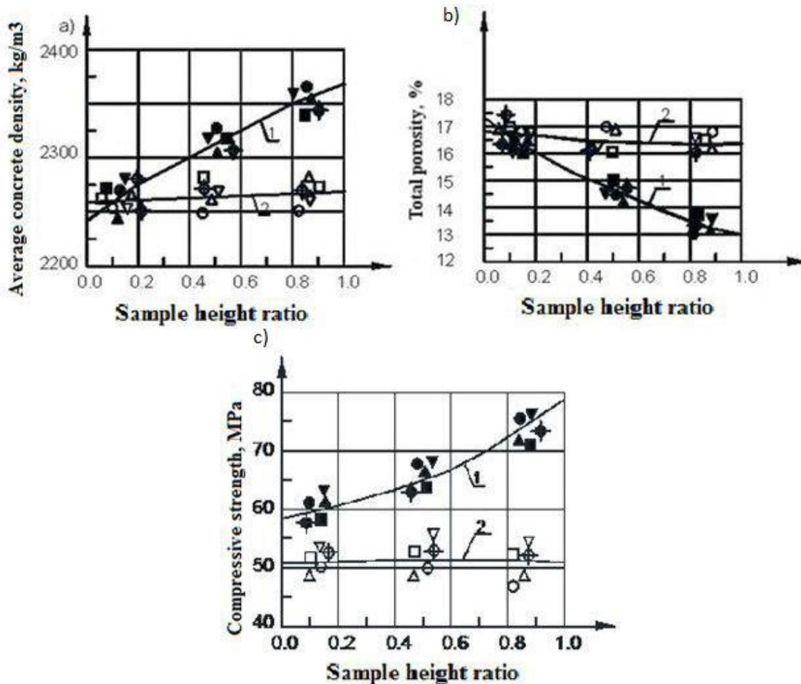
Figure 2. Variance of physical and mechanical properties of concrete along a sample height. (a – average concrete density; b – total porosity; c – compressive strength)
