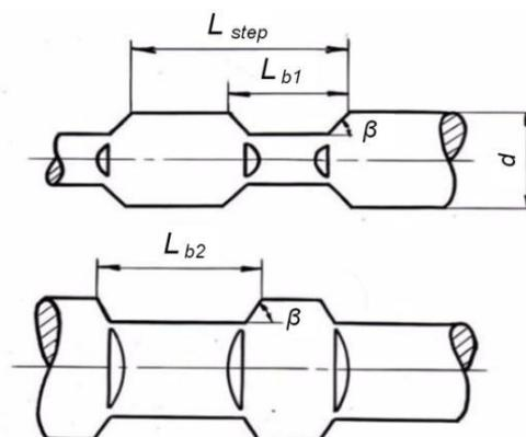
**Figure 3. Scheme of the profile of the fibre in two planes:**
