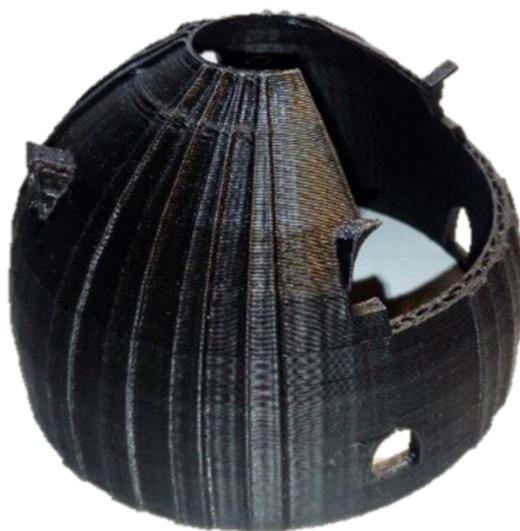
**Figure 1. Dome house model printed on a 3D printer**
