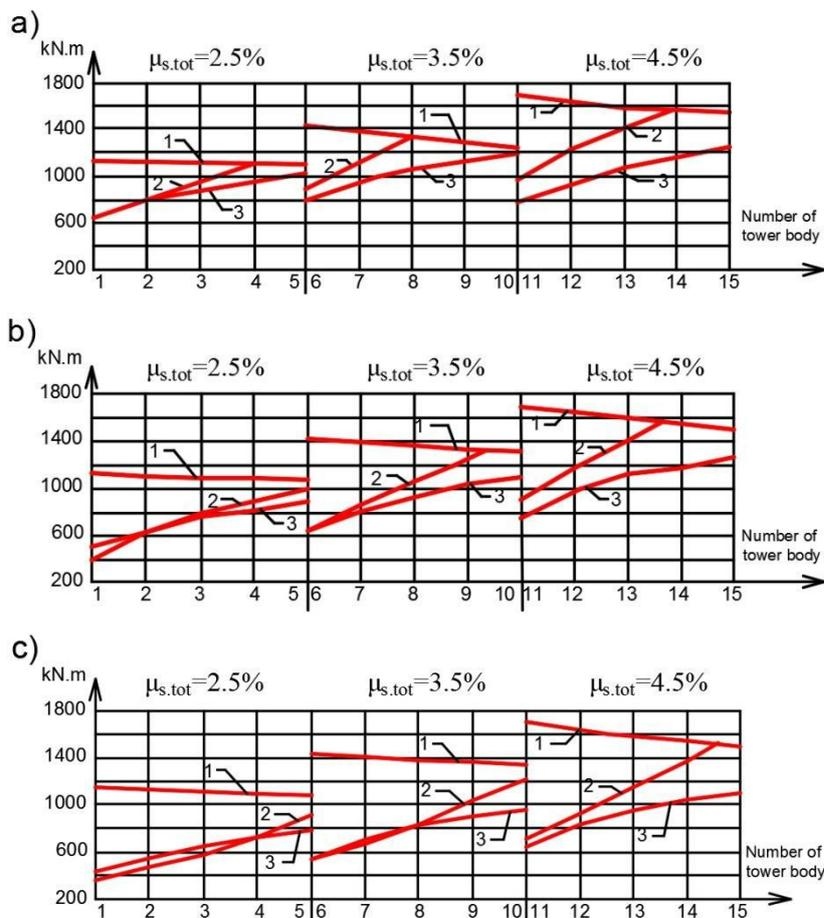
**Figure 4. Changing of bearing capacity of CC20 tower bodies when a)  $MV/M=0$ ; b)  $MV/M=0.2$ ; c)  $MV/M=0.4$**
