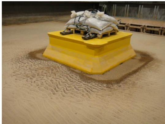
Figure 11. View on BGT model and scour protection (from windward side) after after execution of tests 1a, 1b, 1c, 2, 3 for wave direction with angle 90^\circ to a plane side of BGT "Prirazlomnaja"
