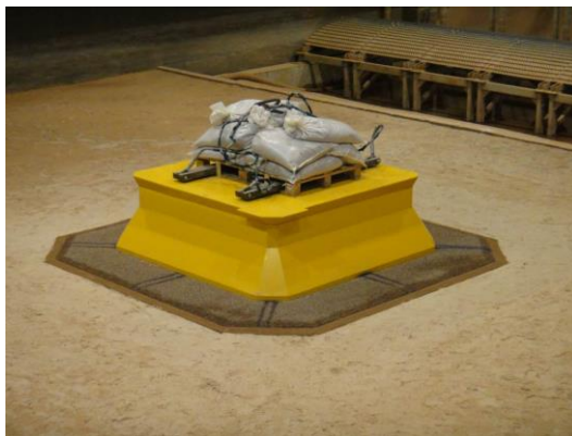
Figure 8. View on BGT model and scour protection before the beginning of experimental researches for wave direction with angle 90^\circ to a plane side of BGT
