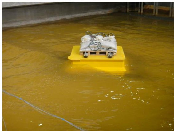
Figure 16. Interaction of waves with BGT during execution of researches for wave direction with angle 45^\circ to a plane side of BGT "Prirazlomnaja" (view from windward side)
