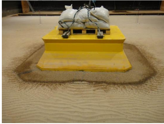
Figure 10. View on BGT model and scour protection (from leeward side) after after execution of tests 1a, 1b, 1c, 2, 3 for wave direction with angle 90^\circ to a plane side of BGT "Prirazlomnaja"
