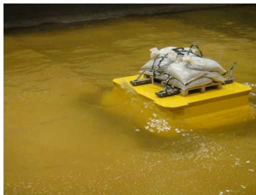
Figure 9. Interaction of waves with BGT during execution of researches for wave direction with angle 90^\circ to a plane side of BGT "Prirazlomnaja" (view from windward side)
