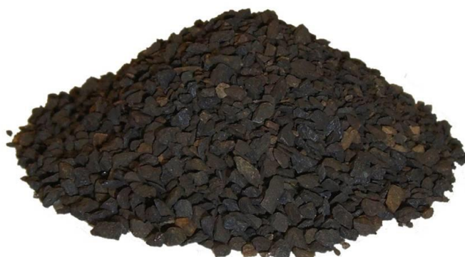
Figure 6 Appearance of the manganese-modified filter-catalyzed materials based on the natural zeolite of the Badinskoye deposit (Russia)
