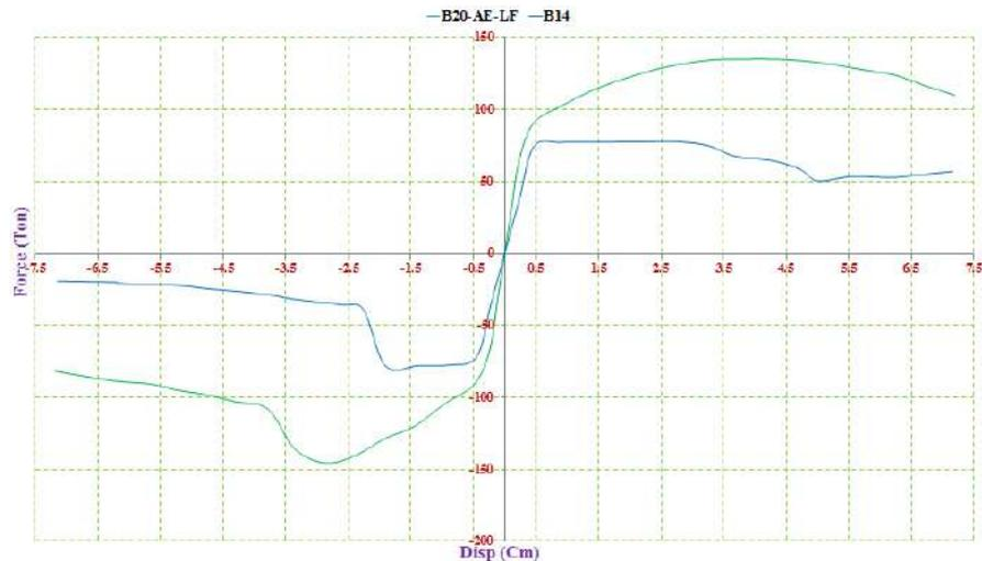
**Figure 11 Comparison between envelope curve of analytical models**
