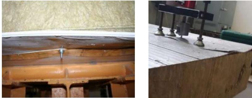
Figures 16 and 17. Delamination of sandwich panel
