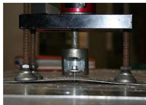
Figure 14 and 15. Process of pulling out a screw (left), hole in the plate after the pull out (right)
