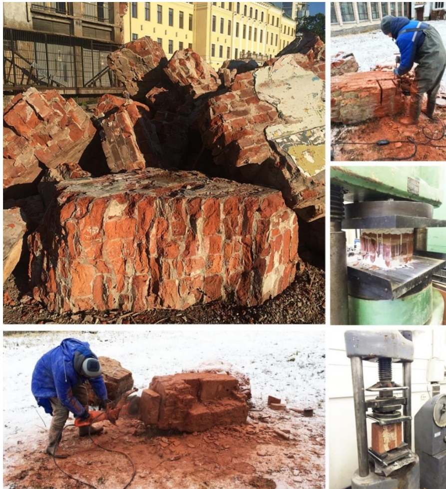
Figure 4. Accumulated brick debris on the demolition plot, prism preparation for compression and shear test and test set-ups
