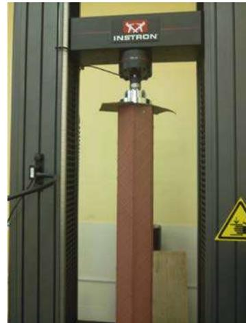
Figure 4. Compression tests of a HWPC sample on Instron 5982 test machine
