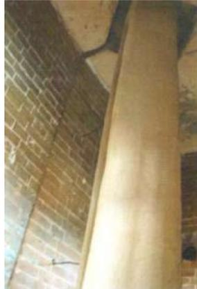
**Figure 4. Appearance of the experimental image of a steel column with a flame retardant "Fendolite MII" after the fire impact (sample No. 1. view of the technological opening of the fire chamber)**
