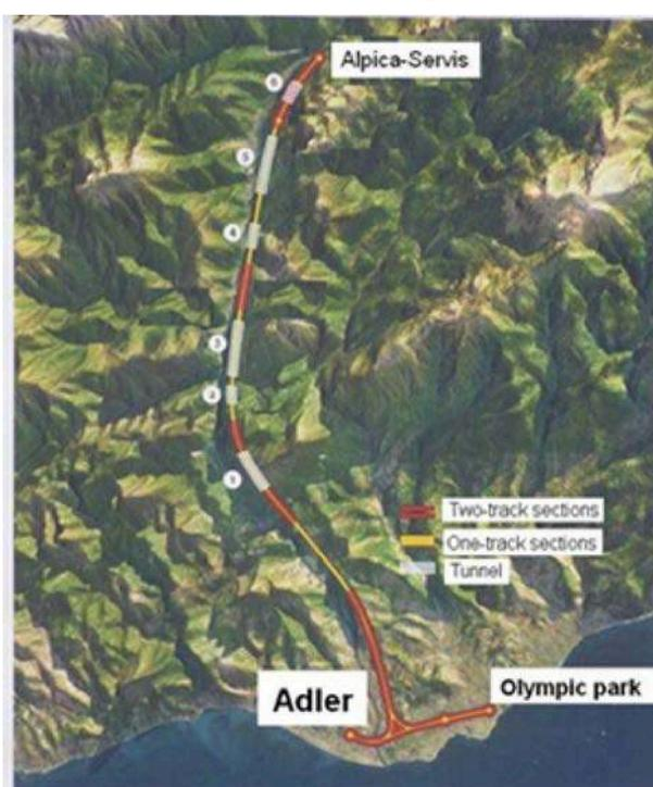
**Figure 1. Tunnel routes layout**
