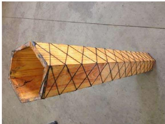
**Figure 1. HWPC sample with external reinforcement in the form of a carbon fiber grid**
