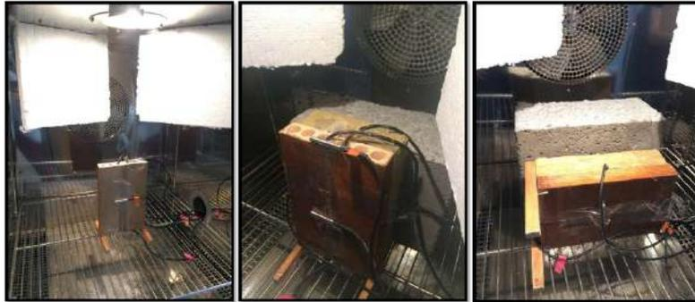
**Figure 5. Different configurations during the trials: (a) without insulation and vertical orientation (d=10mm); (b) with insulation and concrete and vertical orientation (d=15mm); (c) with insulation and concrete and horizontal orientation (d=10mm)**
