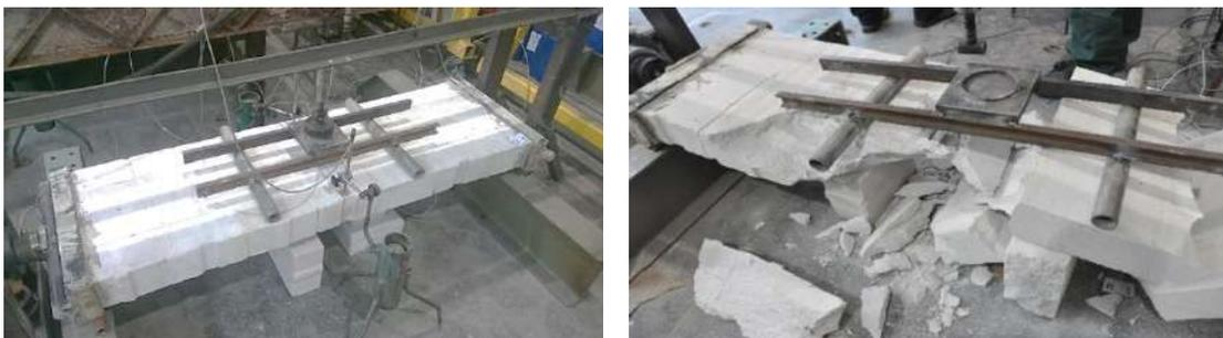
**Figure 3. Type of test specimens during loading and after failure**
