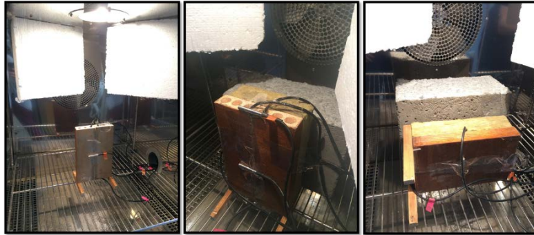
Figure 5. Different configurations during the trials: (a) without insulation and vertical orientation (d=10mm); (b) with insulation and concrete and vertical orientation (d=15mm); (c) with insulation and concrete and horizontal orientation (d=10mm)
