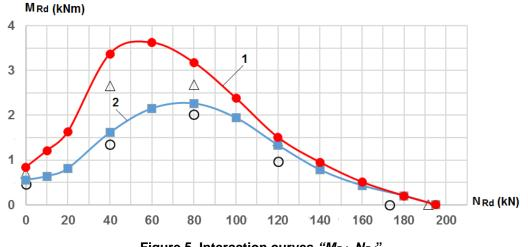
Figure 5. Interaction curves " $M_{Rd}$ - $N_{Rd}$ " 1 – for reinforced specimens; 2 – for unreinforced specimens;  $\Delta$  – experimental values for reinforced specimens;  $\circ$  – experimental values for unreinforced specimens
