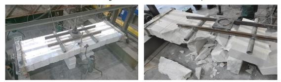
Figure 3. Type of test specimens during loading and after failure
