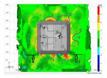
Figure 6. Bottom profile near the Platform model after experiment No. 5:
