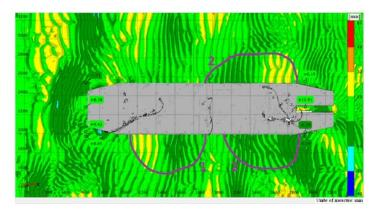
**Figure 9. Bottom profile near the Barge model after experiment No. 7:** 1 – formation of transverse sand waves at the bow parts of the side faces; 2 – formation of transverse sand waves at the stern parts of the side faces
