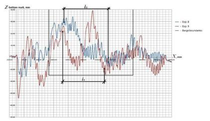
Figure 13. The longitudinal profiles of the bottom surface in cross-section 2-2 along the side of the Barge model as a result of experiments NoNo. 8 and 9
