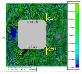
Figure 4. Bottom profile near the Platform model after experiment No. 3: 1 – formation of transverse sand waves at the bow parts of the side faces; 2 – formation of transverse sand waves at the stern parts of the side faces; 3 – formation of transverse sand waves astern of the Platform;
