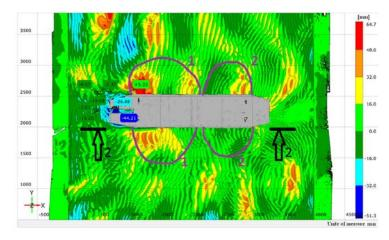
Figure 10. Bottom profile near the Barge model after experiment No. 8:
