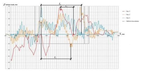
Figure 8. The profiles of the bottom surface along the left side of the Platform in the cross-section 3-3 along the side of the Platform model as a result of experiments NoNo. 2, 3 and 5
