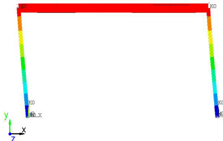
Figure 5. The first buckling mode (plane deformation in face plate). Critical load is 11.2 kN (experimental value). Torsional stiffness of beam-pillar connection with regard to the rotation about z-axis is 2820 N-m/rad
