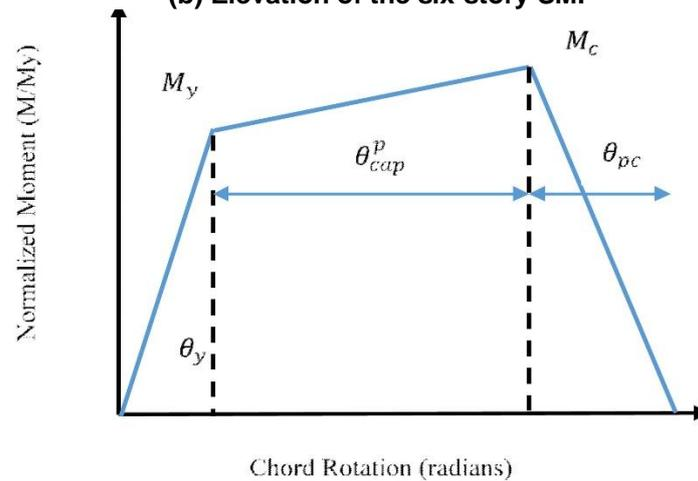
Figure 2 Monotonic behavior of component model used to model reinforced concrete beam-column elements [8]
