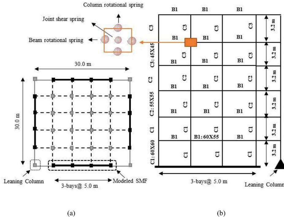
Figure 1 (a) Typical plan view of the concrete structure model and (b) Elevation of the six-story SMF
