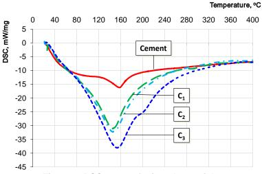
Figure 1. DSC curve of mineral materials
