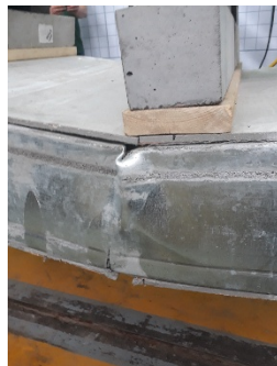
Figure 9. The destruction in the "dangerous" section
