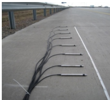
Figure 2. One set of temperature and moisture sensors
