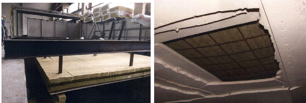
Figure 5. A sample of the ceiling design before the test (left) and partial collapse of the enclosing part of the suspended ceiling during cooling (right)
