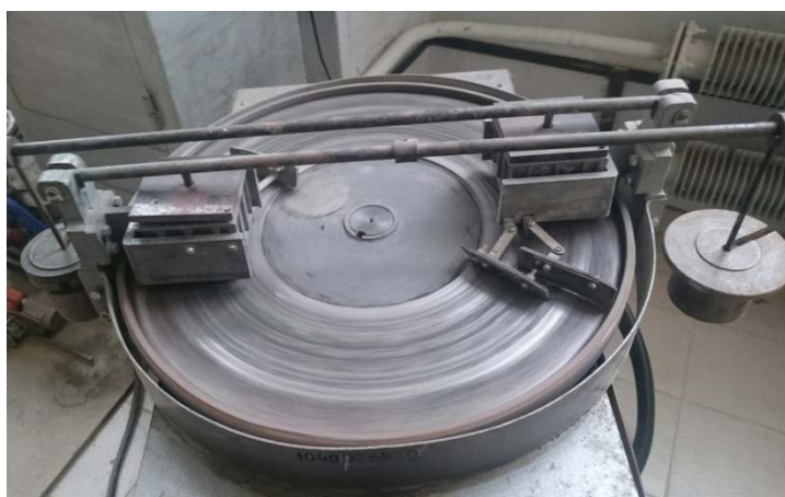
Figure 2. Testing the fiber samples for abrasive capacity (abrasive wear).
