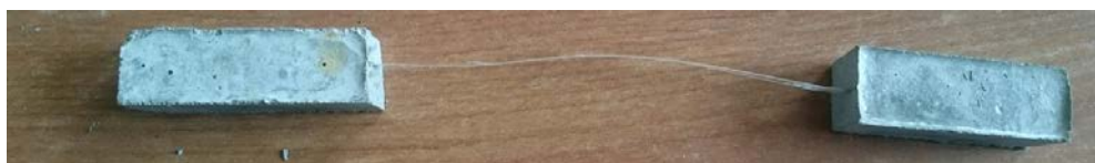
Figure 3. A sample for testing the fiber adhesion strength with the concrete matrix (determination of the critical length of the fiber).
