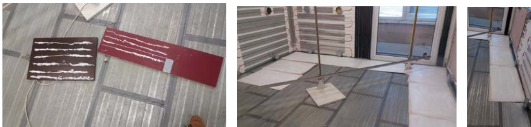
Figure 1. Pictures showing how the pollution sources - acrylic based hermetic sealant (left side); waterborne acrylic-based paint (middle) and solvent based paint (right side), were applied.
