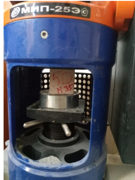
Figure 2. The sample in the compression apparatus.
