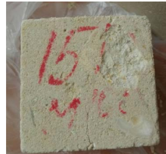
Figure 6. Cracks on the untreated sample.
