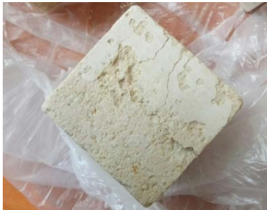
Figure 5. Cracks and delamination on the untreated sample.
