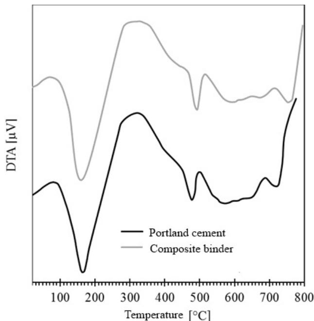
**Figure 4. DTA results for pure cement stone and cement stone of the CB.**
