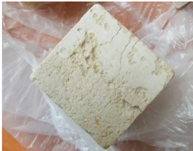
Figure 5. Cracks and delamination on the untreated sample.
