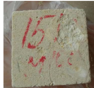
Figure 6. Cracks on the untreated sample.
