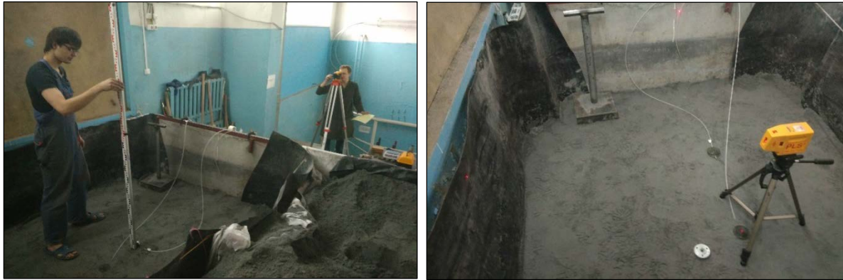
Figure 2. Sensor positioning in the ash and slag mixture body.
