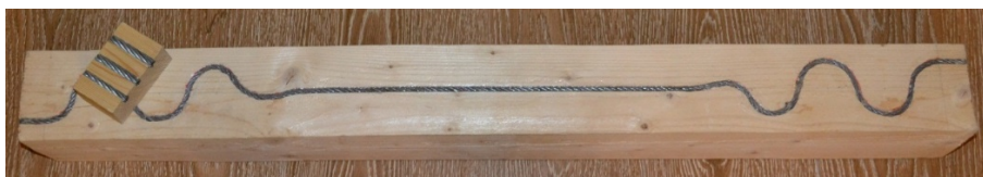
Figure 2. Demonstration samples of reinforcement along a curvilinear path
