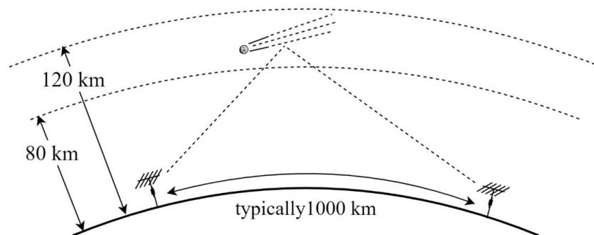
Fig. 1. Illustration of the principle of MBC [2]
