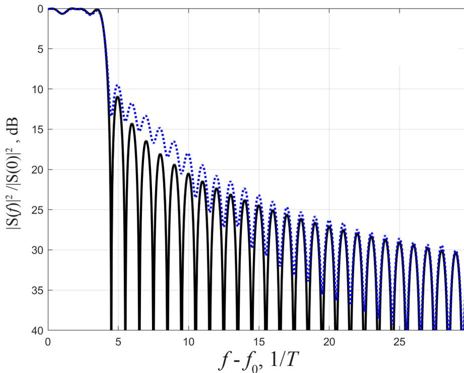
Fig. 7. Energy spectrum of signals at different values of PR
