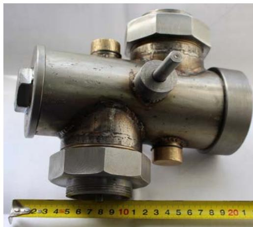
**Figure 3. Pulsed flow distributor.**
