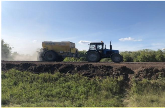
**Figure 9. Cement spreader – semi-trailer van Bomag BS12000.**
