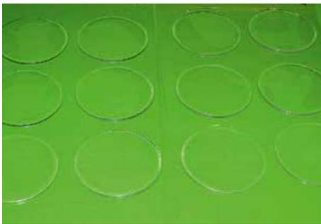
Figure 1. Silicone film of a thickness of 1 mm [21].
