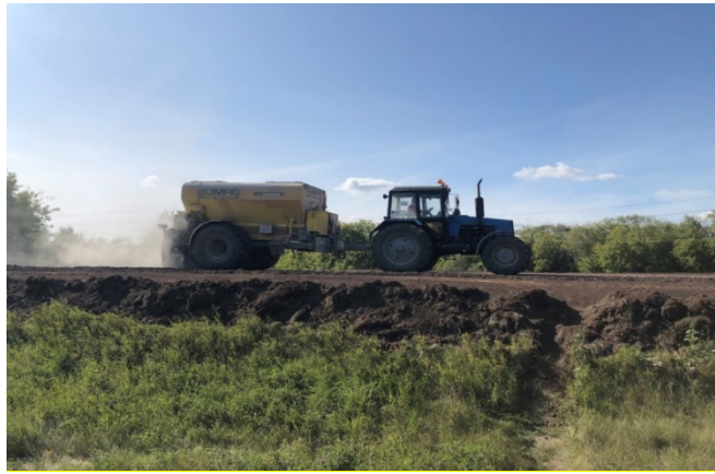
Figure 9. Cement spreader – semi-trailer van Bomag BS12000.
