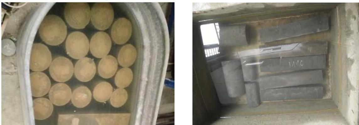
**Figure 2. Moistened the sample after casting.**
