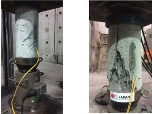
**Figure 8. Experiment to determine stress – deformation.**
