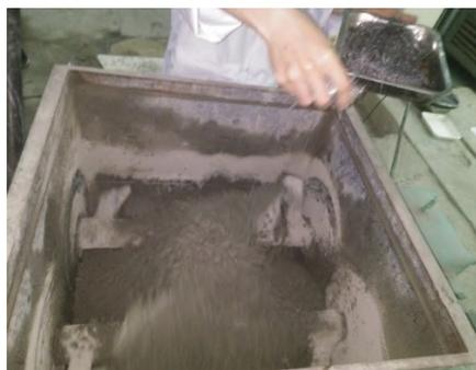
**Figure 10. Mixing nano-concrete mixture with steel fibers.**
