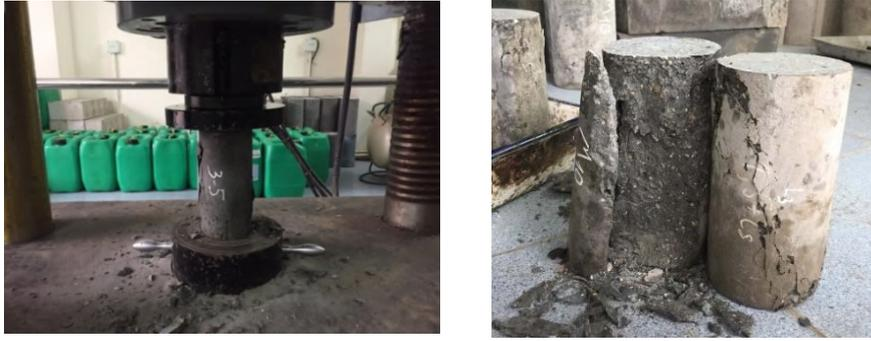
**Figure 3. The sample is destroyed during the compression.**
