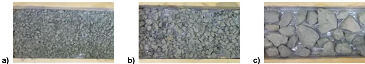
**Figure 1. Granite pieces with different dimensions joined with the timber board by the epoxy glue: (a) 2-5 mm; (b) 5-8 mm; (c) 16-25 mm [19]**
