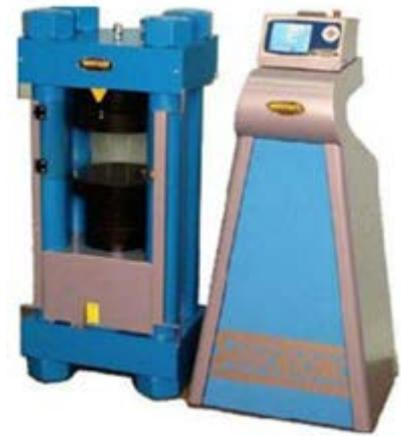
Figure 6. Machine for strength tests, MATEST E160.
