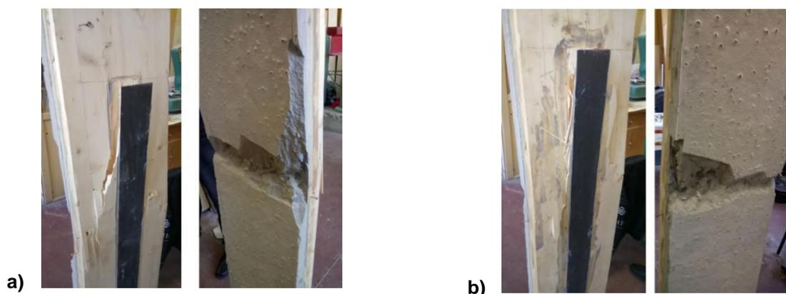
**Figure 8. The failure mode for the specimens from the first and second sub-groups: (a) second specimen; (b) fourth specimen [19]**
