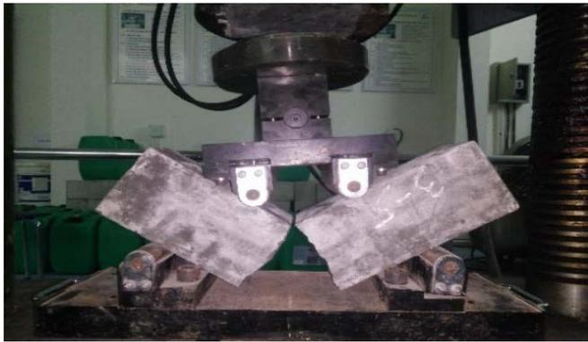
**Figure 5. Tensile strength test when bending.**
