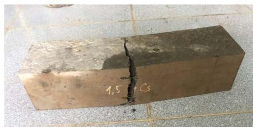
**Figure 11. 4-point bending test and sample after destructive.**
