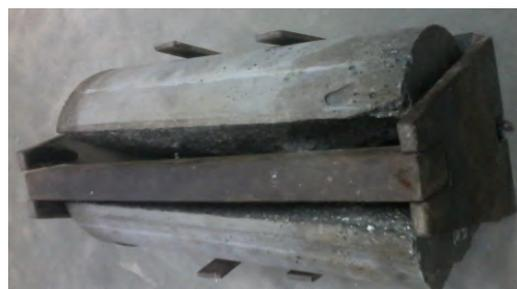
**Figure 7. Test strength of splitting.**
