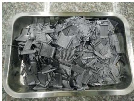
**Figure 1. Dramix steel fibers used in research.**
