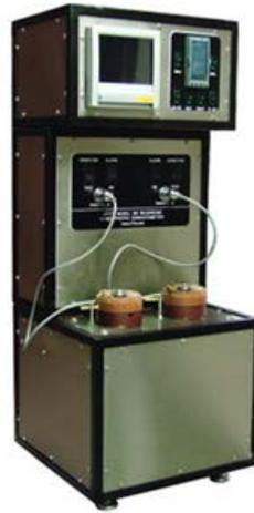
Figure 5. The atmospheric pressure consistometer, OFITE 80.
