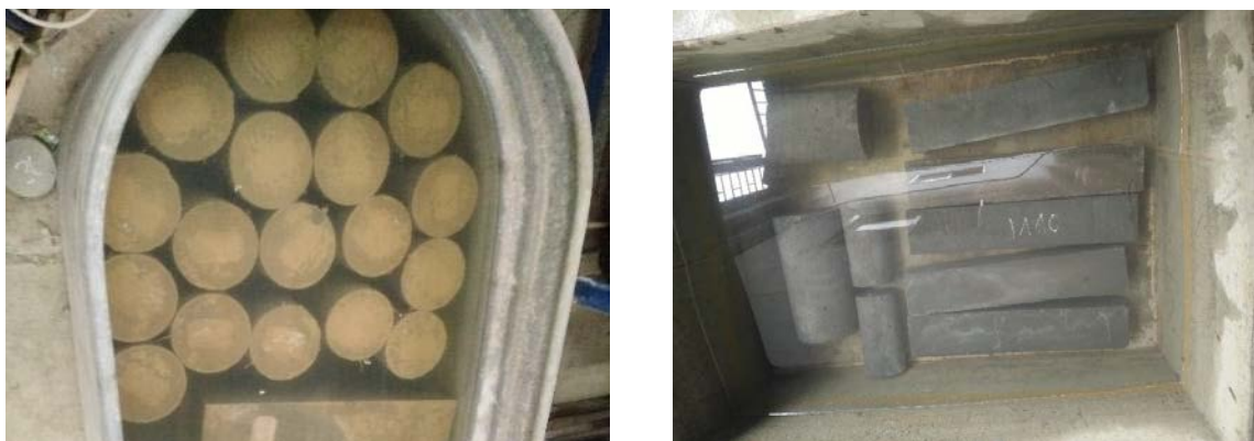
Figure 2. Moistened the sample after casting.
