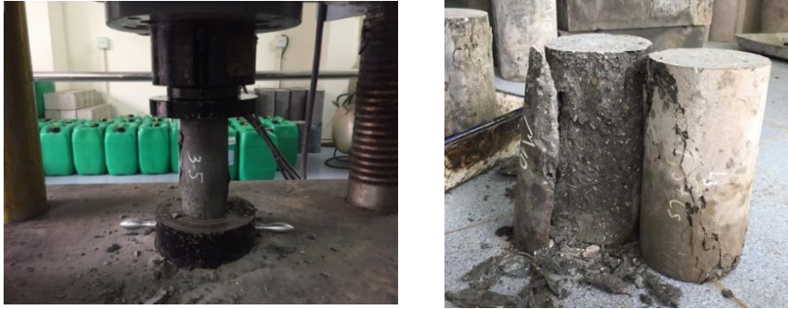
Figure 3. The sample is destroyed during the compression.
