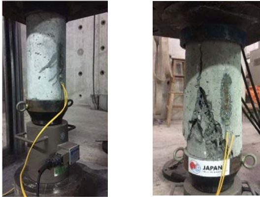
Figure 8. Experiment to determine stress – deformation.
