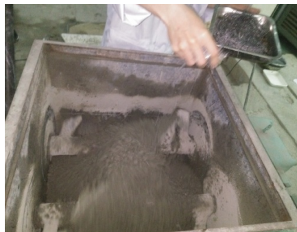
Figure 10. Mixing nano-concrete mixture with steel fibers.
