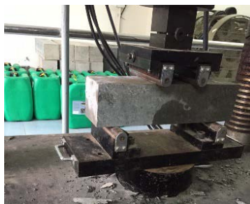
Figure 11. 4-point bending test and sample after destructive.
