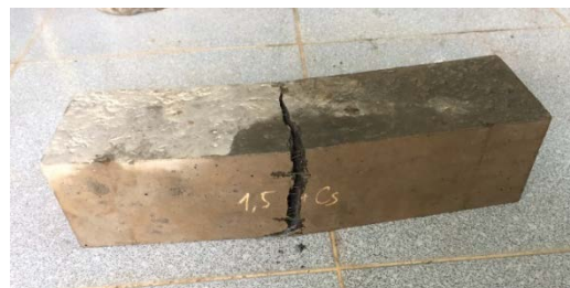
Figure 11. 4-point bending test and sample after destructive.
