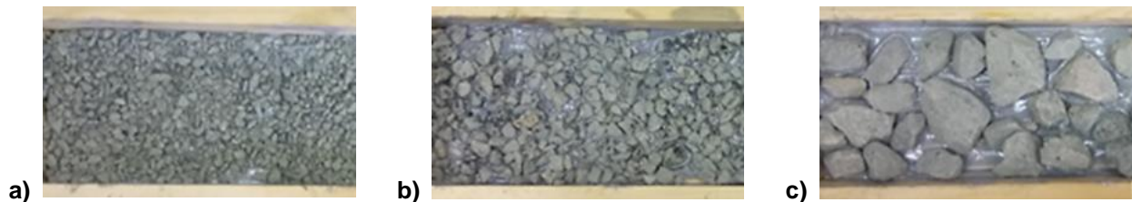
Figure 1. Granite pieces with different dimensions joined with the timber board by the epoxy glue: (a) 2-5 mm; (b) 5-8 mm; (c) 16-25 mm [19]
