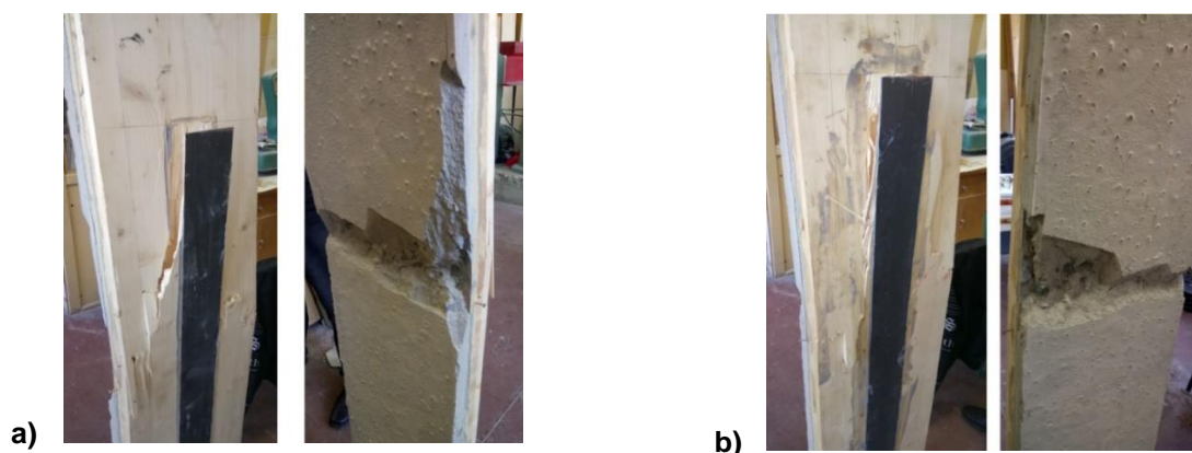
Figure 8. The failure mode for the specimens from the first and second sub-groups: (a) second specimen; (b) fourth specimen [19]
