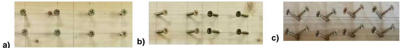
Figure 2. Considered variants of screws placement: (a) screws were placed under the angle 90° relatively to longitudinal axis of the specimens; (b) screws were placed under the angles 45°; (c) two screws were placed in each point under the angle 45° [19]
