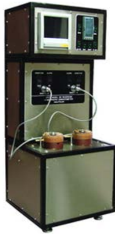
Figure 5. The atmospheric pressure consistometer, OFITE 80.
