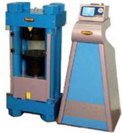
Figure 6. Machine for strength tests, MATEST E160.
