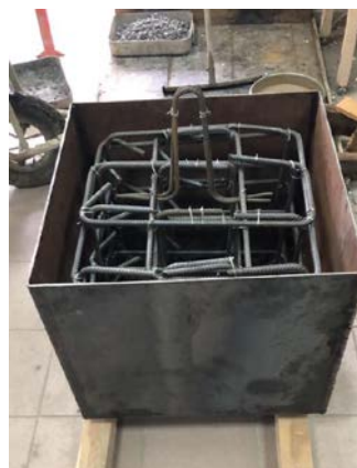
Figure 4. RC block reinforcement (cm).
