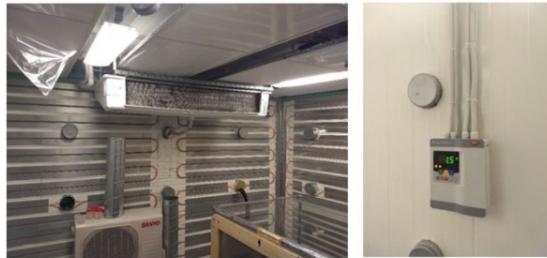
Figure 2. The cooling device, which ensured simulated outdoor air temperature in the climatic chamber.
