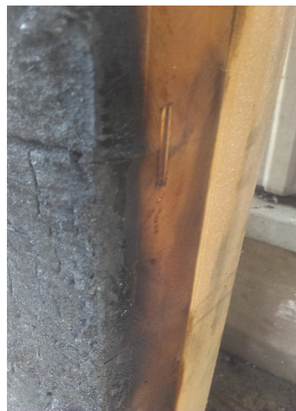
Figure 7. Development of foamed coil after the testing of sample 7.
