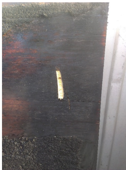
Figure 7. Development of foamed coil after the testing of sample 7.
