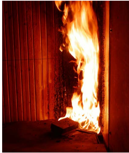
Figure 6. Sample 4 – bloating of the lacquer.
