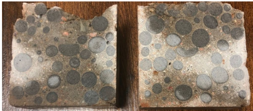
Figure 2. A section of the concrete cube after compression test.
