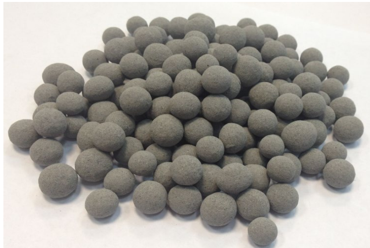
Figure 1. Cold-bonded fly ash aggregate used in the experiment.
