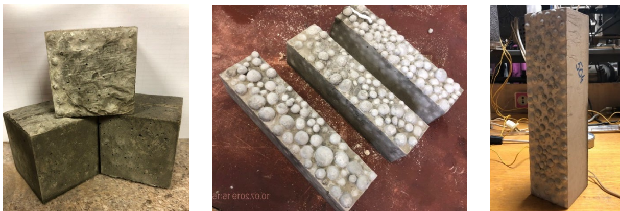
Figure 3. Cold-bonded fly ash aggregate concrete specimens.
