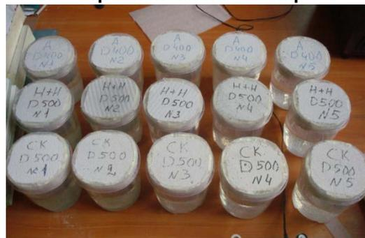
Figure 4. Determination of vapor permeability of samples.
