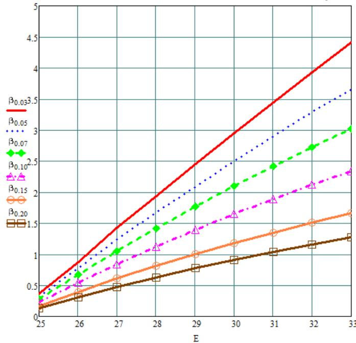
**Figure 2.  $\beta - E[E]$  diagrams at the different levels of variation coefficients for pile material elastic modulus  $E$ .**
