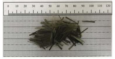
Figure 2. Basalt fiber.
