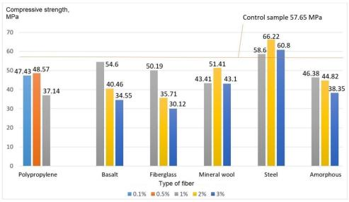
Figure 9. Compressive strength test results of fiber-reinforced concrete specimens.
