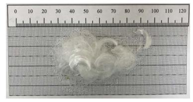
Figure 1. Polypropylene fiber.
