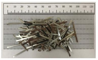
Figure 6. Amorphous fiber (Fe-B-C system).
