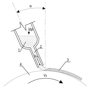
Figure 7. Scheme of the spinning process. 1 – molten metal, 2 – jet of melt, 3 – amorphous metal fiber, 4 – cold drum
