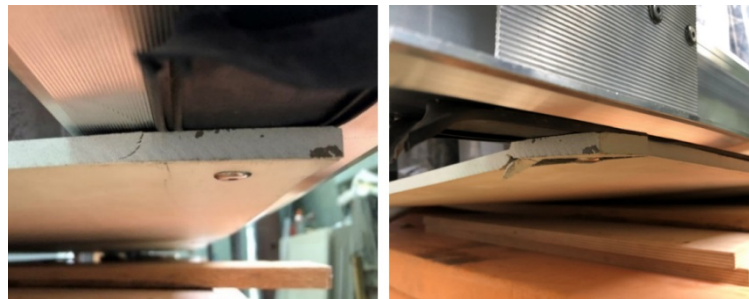
Figure 17. Left – the formation and opening of a crack in sample 5 under the load of 266.67 kg/m 2 ; right – corner fastening point after the panel fracture.
