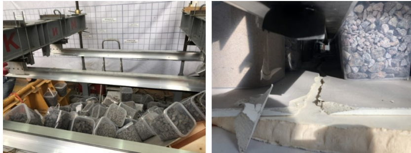
Figure 16. Fracture of the panel: left – sample 3 under the load of 222.22 kg/m 2 ; right – sample 4 under the load of 200 kg/m 2 .
