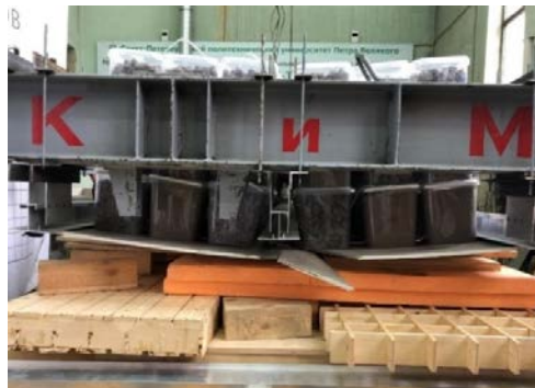
Figure 18. Panel fracture of the sample 5 under the load 344.44 kg/m 2 .
