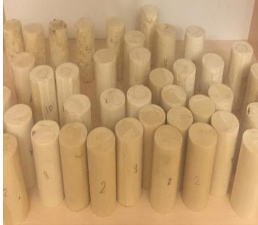
**Figure 4. The prepared resin's samples of different densities.**
