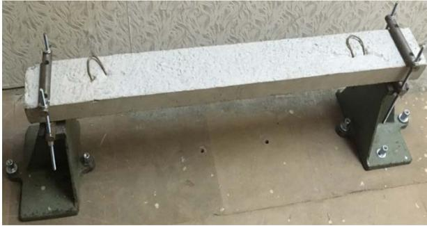
**Figure 4. Fixing the test sample on the stand.**
