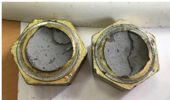
Figure 19. Fracture surfaces of severed bolt heads.
