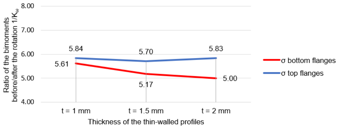
Figure 8. Dependence graphs of the bimoment change on the thin-walled profiles thickness for the rigid joint.
